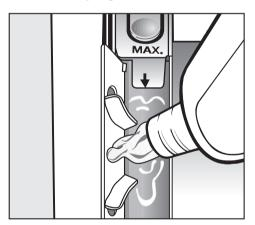
Add the fabric conditioner or liquid starch to compartment %. Do not exceed the maximum level mark.
